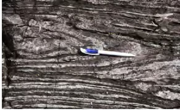
Figure 1: Banded Iron Formation with the dark ore being magnetite and the white being silica (Quartz). This photo is of the BIF observed at the AKORA Resources Traramarina project. Source: AKORA.
