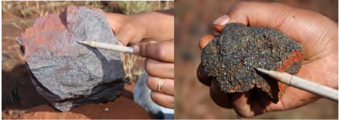
Figure 2. Typical iron ore rocks; left is Hematite and the right is Magnetite.
