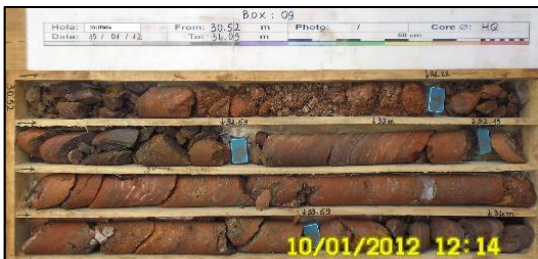
Photo 8.5: Hematitic Material in DD12004
