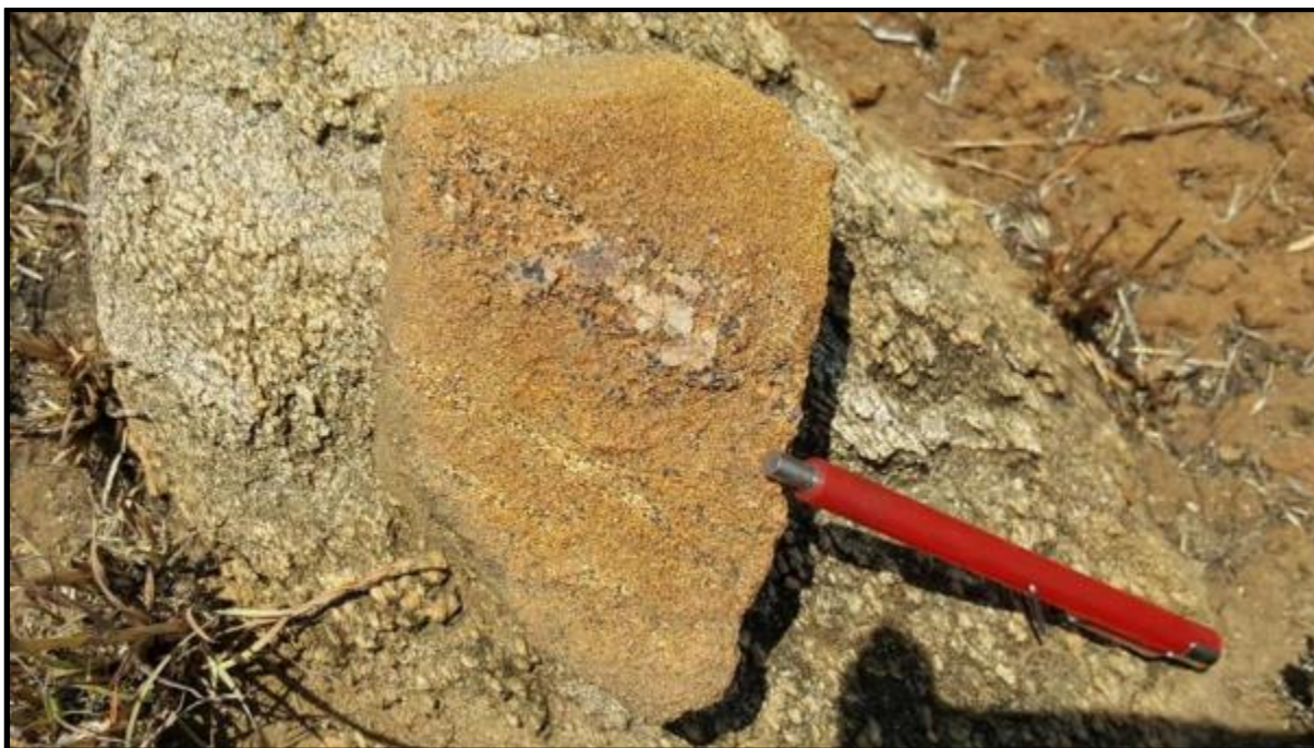
Photo 7.9: Magnetite Bearing Quartzite East of Main Iron-Ore Target
