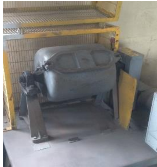
Photo 12.4: Bond Ball Mill Test Equipment
