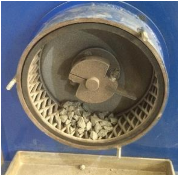
Photo 12.3: Bond Abrasion Test Equipment
