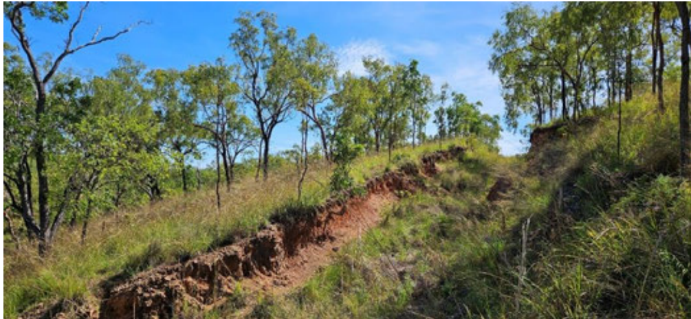
Figure 5-4: Costean thought to date from 1980s on Mt Wandoo (located across sample points WAT 7-1 to WAT 7-15)
