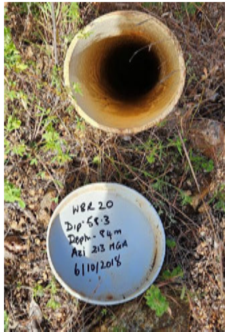
Figure 5-9: Example drill hole with cap and details
