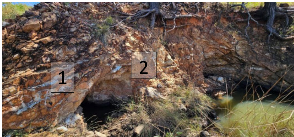
Figure 5-5: Historic mining shaft thought to have been reworked with an excavator in the 1990s showing kaolinite spoil to the east (right of frame)
