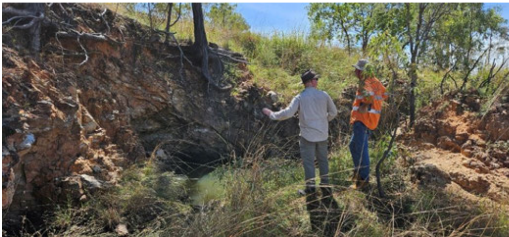
Figure 5-5: Historic mining shaft thought to have been reworked with an excavator in the 1990s showing kaolinite spoil to the east (right of frame)
