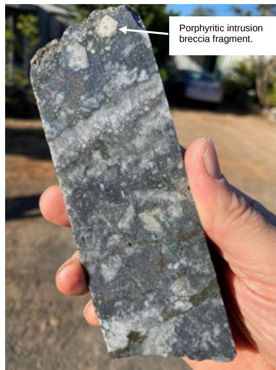
Sulphide "D vein" in Dingo diamond core: part of 3m at 0.4 g/t Au and 150 g/t Ag, 0.25% Sb fr 61m
