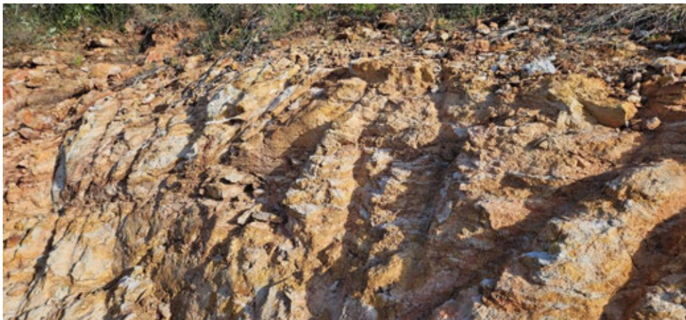
Figure 5-8: Sub-horizontal fractures visible in drill bench (bench containing WBR069)
